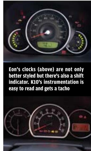
Eon's clocks (above) are not only better styled but there's also a shift indicator. K10's instrumentation is easy to read and gets a tachometer
